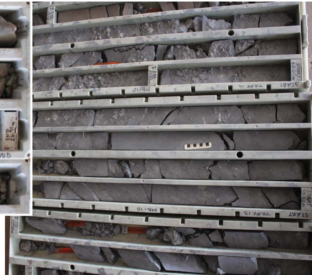
Image: HQ diamond core – Graphite Schist from Drillhole MD-13 - Mount Dromedary. Photo courtesy of F. Von Gnielinski, GSQ, 2016.
