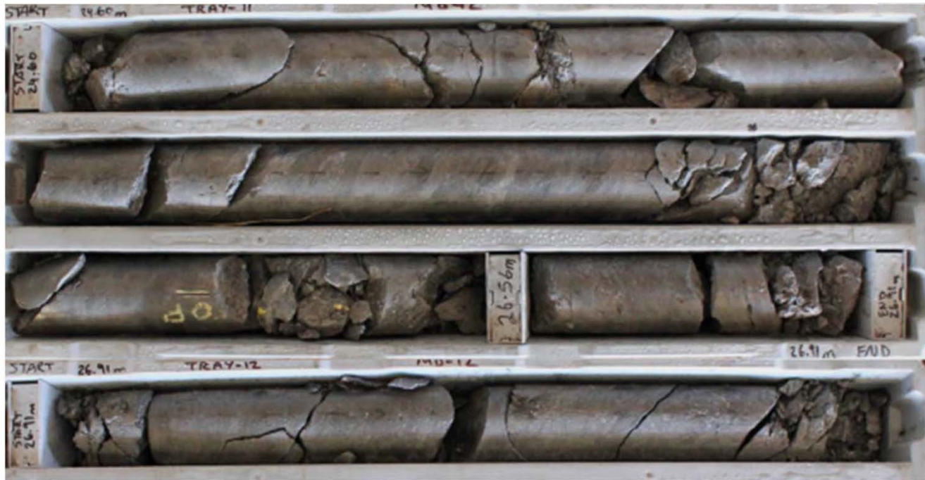
Image: HQ diamond core – Graphite Schist from Drillhole MD-12 - Central Zone of the Mount Dromedary December 2015.
