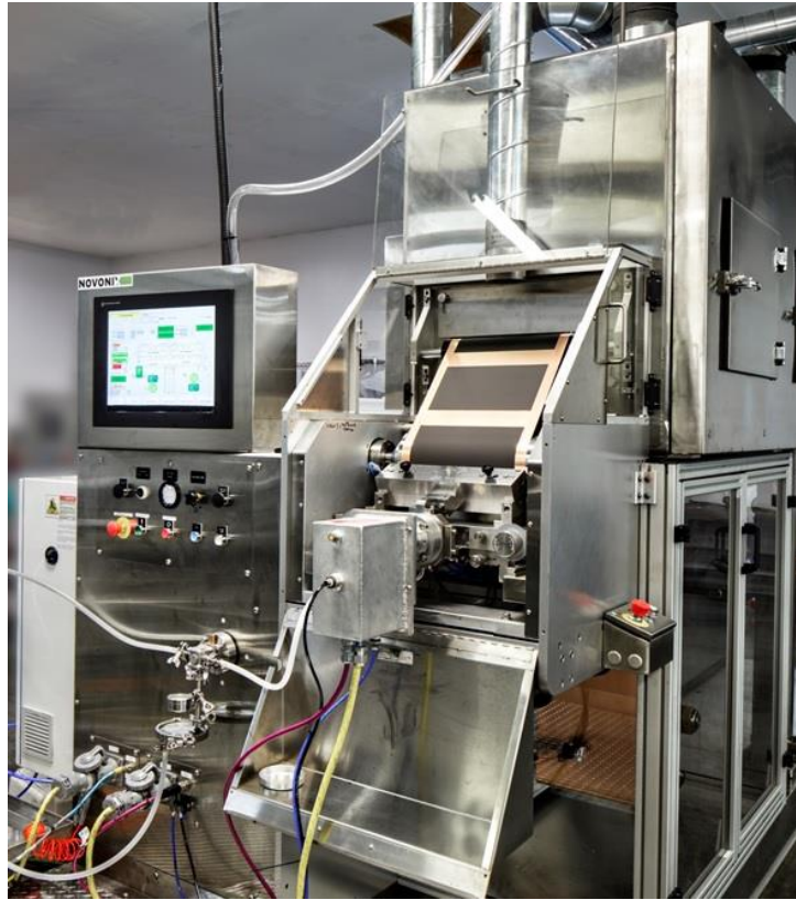
Photo: Professor Jeff Dahn of Dalhousie University with Dr Chris Burns NOVONIX COO inspecting the electrode slitting operation at the NOVONIX battery cell manufacturing facility
