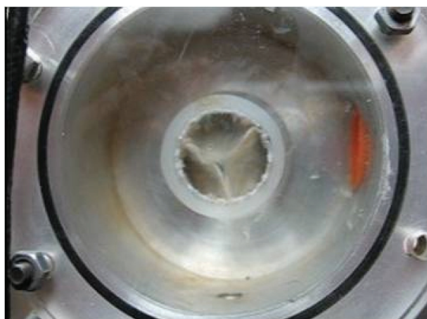
Kangaroo pericardium being tested on the pulse duplicator
