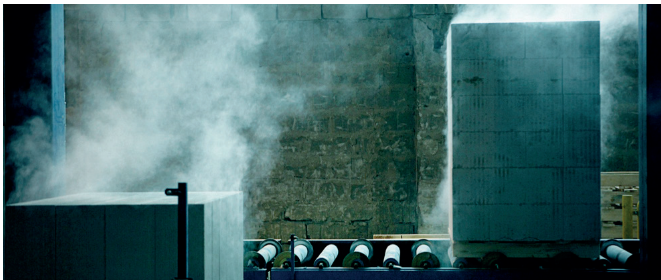
Autoclave transfer cars and autoclave modification works. during the second quarter of 2018 to reach normal production by the end of the second quarter.
