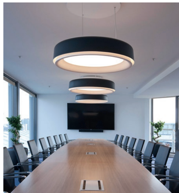
Tinby moulds this top reflector and outer shade for Louis Poulsen 'LP Grand' in solid PUR
