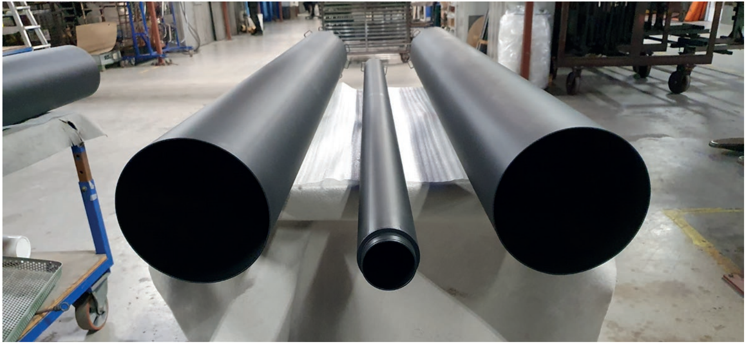
Pipes coated with P153 – a coating for non-stick and low-friction applications
