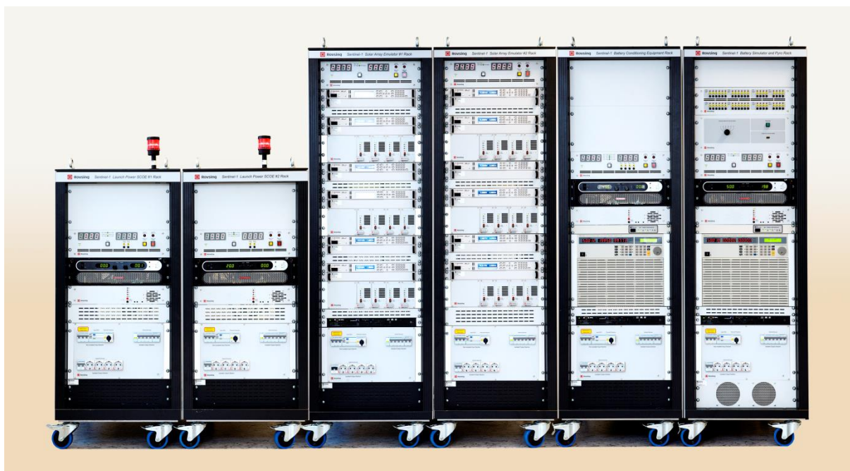
Sentinel 1 Power SCOE System
