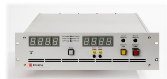
Satellite Launch Power Platform
