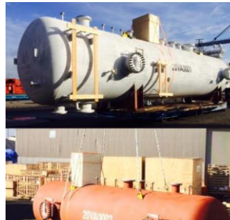
Inlet and test separators
