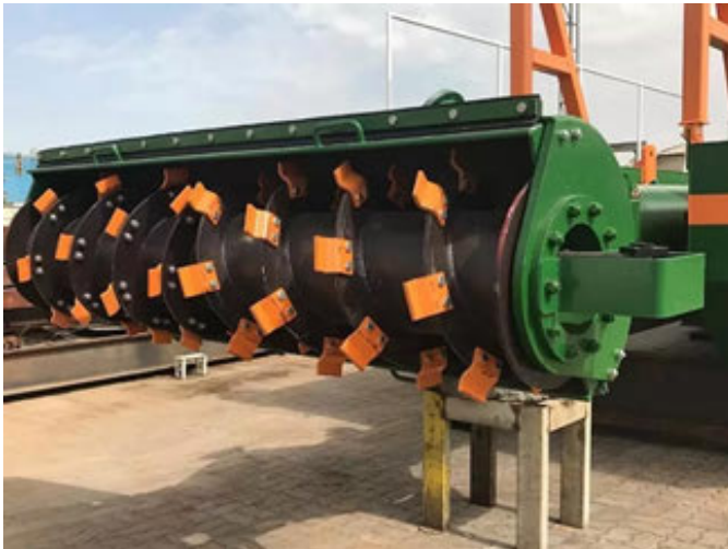
Figure 1: Example of auger dredger with a retractable visor which closes around the auger when dredging to prevent particles from spreading. Source: www.dredgeyard.com
