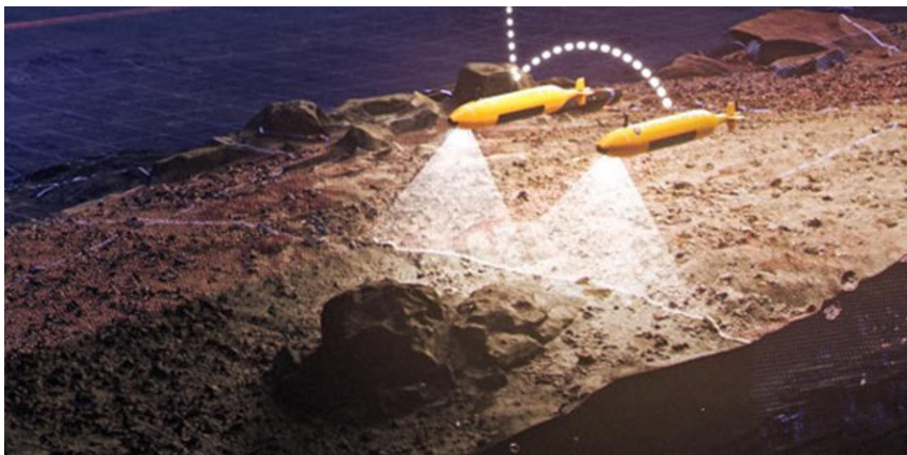
Figure 1. Autonomous deep sea marine mineral exploration surveys using a variety of sensors. Fusion of high-resolution acoustic sonar data with data from a specifically tailored Controlled Source EM (CSEM) system on-board the AUVs enhances the interpretation and classification of the seafloor and near seafloor.
