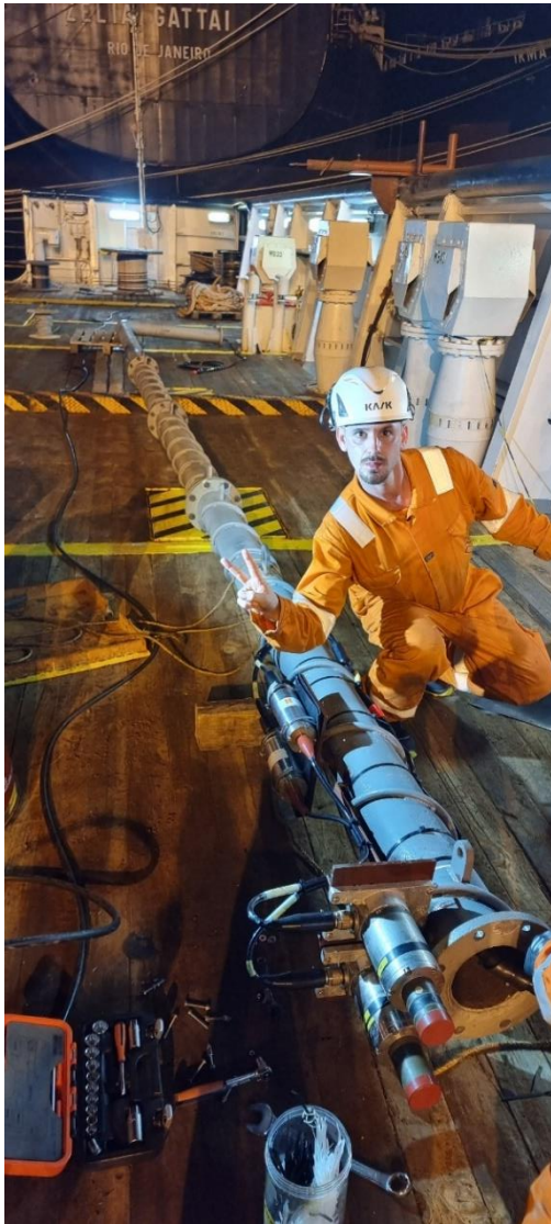
Argeo crew installing Hugin subsea communication system
