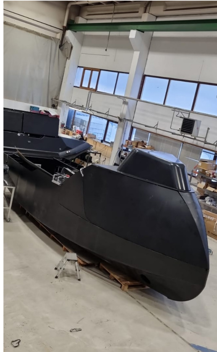
First USV with X-Bow design
