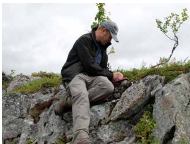
Measuring magnetic susceptibility on Rönnbäcken outcrops.
