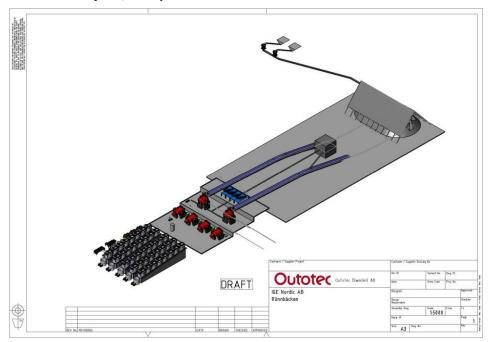
The conceptual concentrator design is derived from a conventional flowsheet, similar to that in other operations which successfully treat disseminated low-grade nickel sulphides. This design, together with capital and operating cost estimates for the concentrator, has been prepared by Outotec AB (Sweden). The mill would have a capacity of 30 million tonnes per annum or 3,750 tonnes per hour, and would produce approximately 95,000 tonnes per annum of nickel concentrate at 28% nickel.
