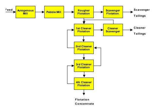
Follow-up laboratory-scale testwork based at Outotec has indicated that concentrates with an increased grade of 28% nickel at 80% sulphide nickel recovery could be produced from the same composite samples used in the minipilot operation. This grade was realised by introducing a new combination of flotation variables, most significantly a new reagent regime, along with slight changes to the flowsheet and, typically, a primary grind of  $P_{80}$  50µm.
