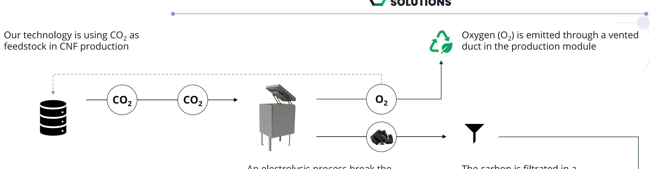
An electrolysis process break the chemical bonding. Carbon (C) can then be taken out of the production module and transferred manually over to the filtration module
