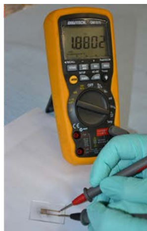
Pristine Graphene resistance 1,700 – 1,900 Ohm
