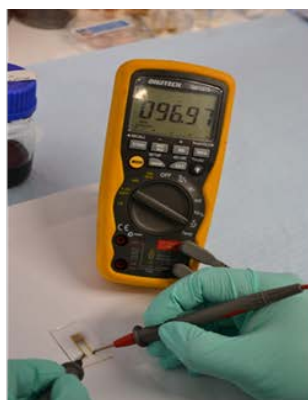
FGR Large area graphene resistance <100 Ohm
