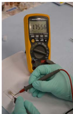
Pristine Graphene resistance 1,700 – 1,900 Ohm
