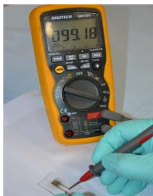
FGR Large area graphene resistance <100 Ohm
