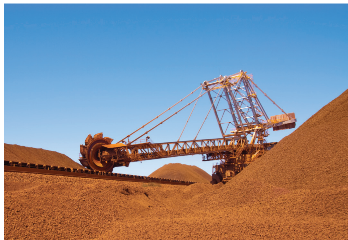
Fig. 1 - Typical Sandvik 12,000 tph bucket-wheel reclaimer.
