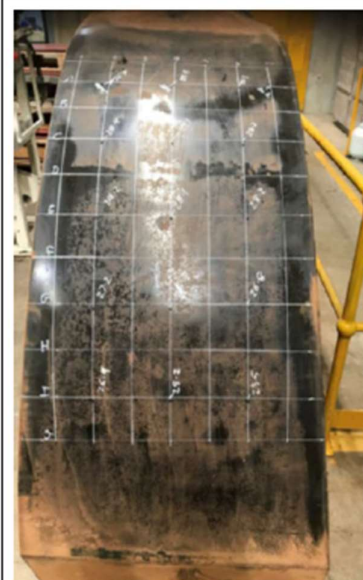
Fig.2c): ArmourGRAPH™ Liner After 62 weeks.
