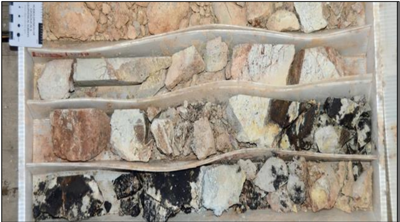
Figure 7-5. Mineralization textures, types at Dios Padre.
