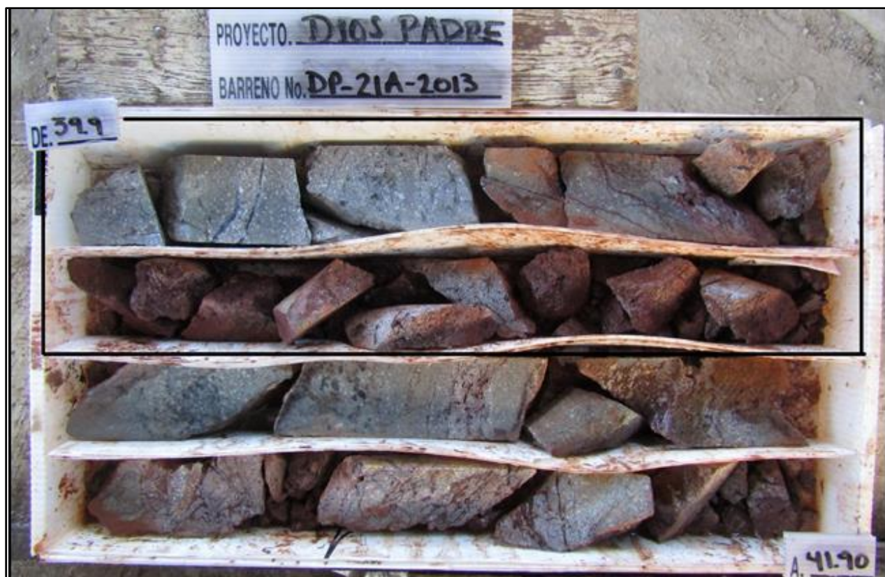
DP 21A -2013 39.5 – 41.9 m, 780 g Ag Breccia 1- stockwork, micro-fractures in rhyolite, note re-healed textures.
