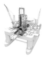
WOR on a semisub for subsea wells
