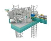
WOR on a jack up for P&A and workover operations
