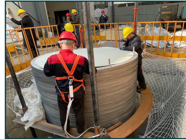
Cell stacking at the fabrication facility in Tianjin, China
