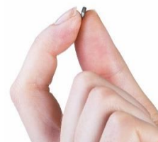
The planned Sencell dimensions are 2*3*6 mm 3
