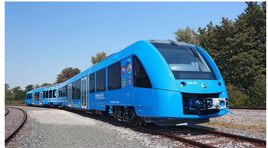
Coradia iLint – world's first hydrogen train launched by ALSTOM during InnoTrans in 2016
