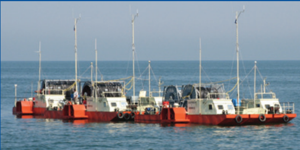
Purpose built vessels for shallow water and transition zone 2D and 3D operations in the Caspian Sea.
