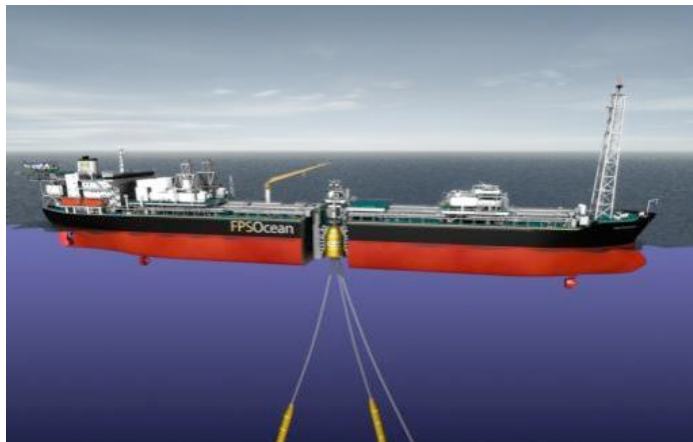
Loading system for FPSOs
