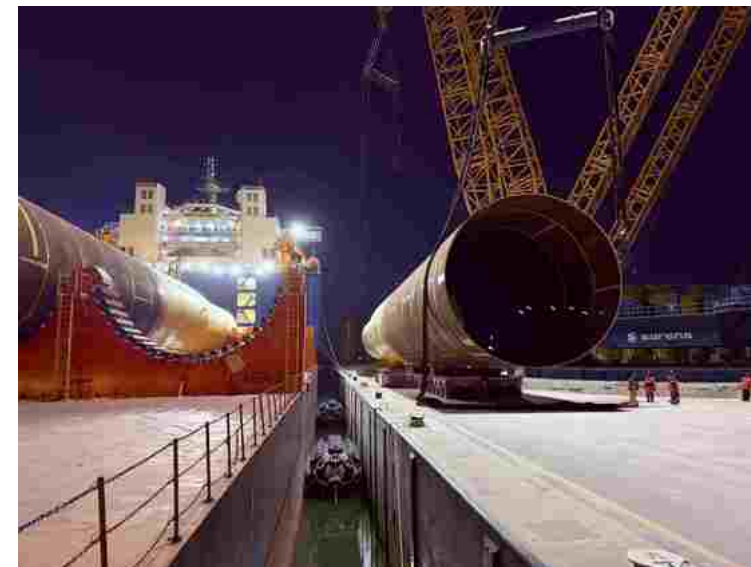
picture: load-out of monopiles for Empire Wind 1
