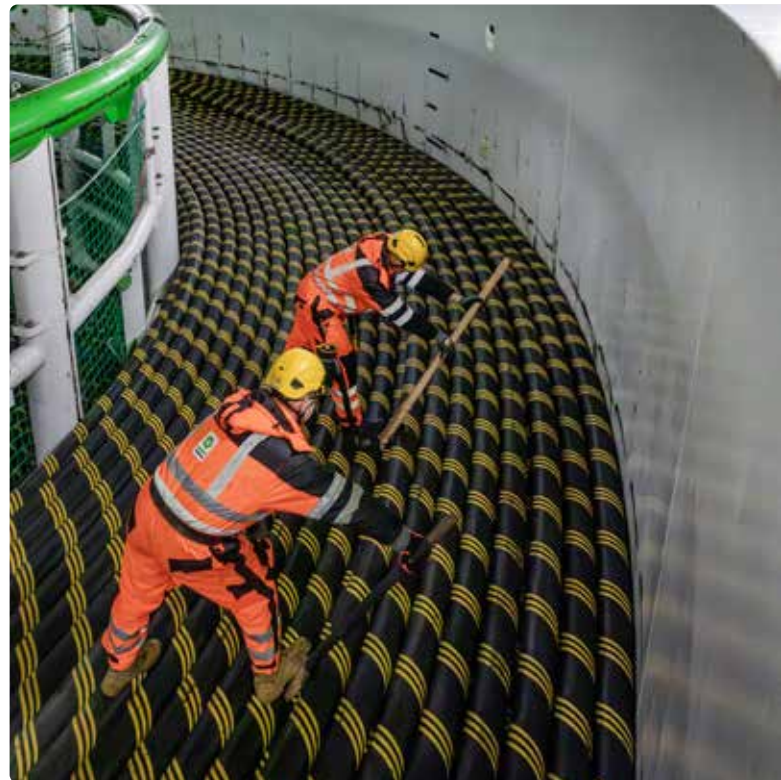
DEME • Cable-laying vessel 'Viking Neptun'
