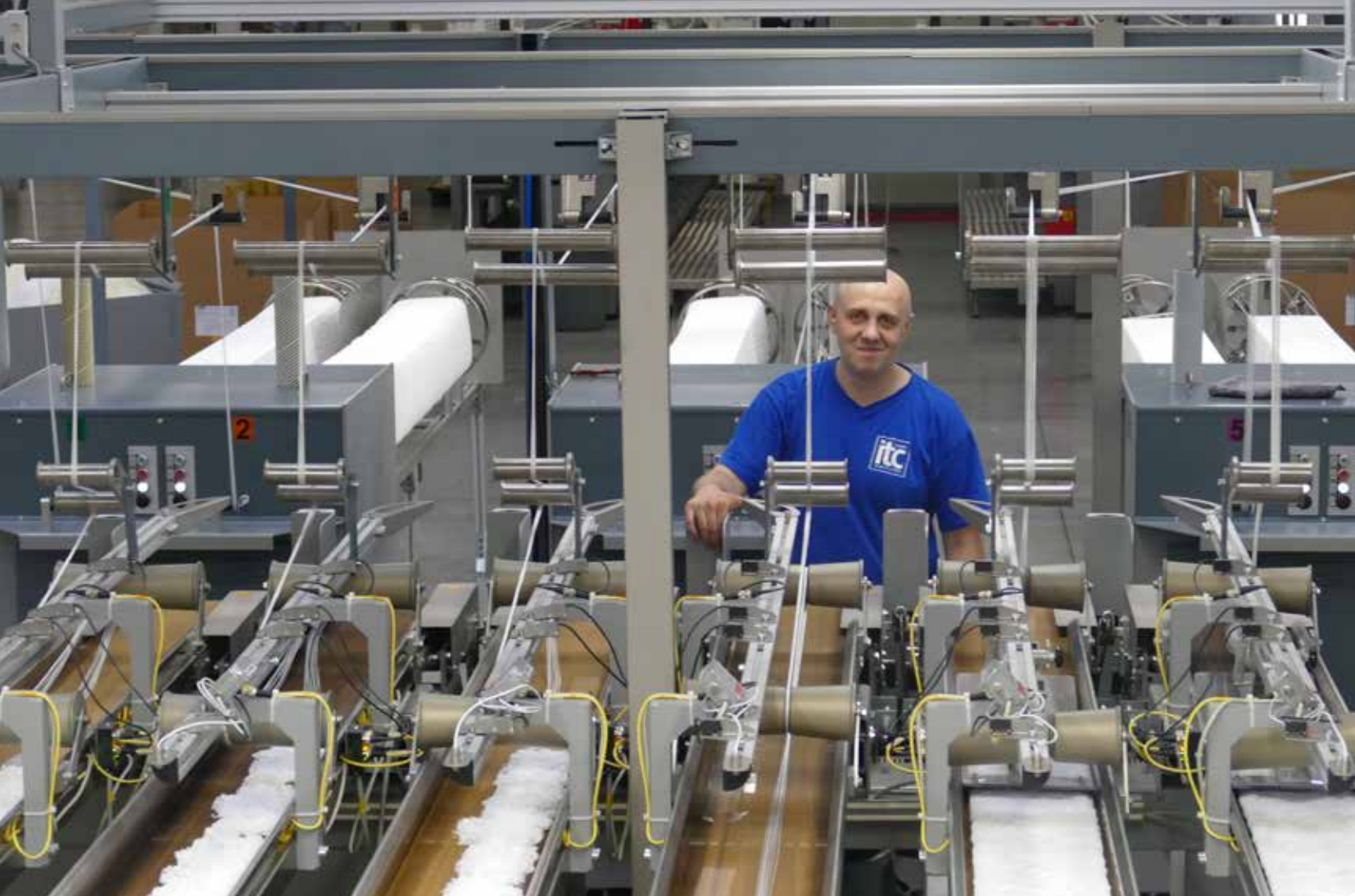
Heatsetting nylon yarn in Balta Tiel
