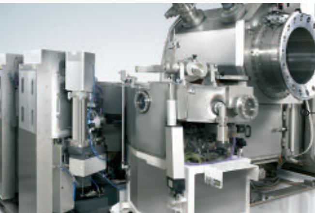
New TIMARIS PVD cluster tool for MRAM wafer under construction
