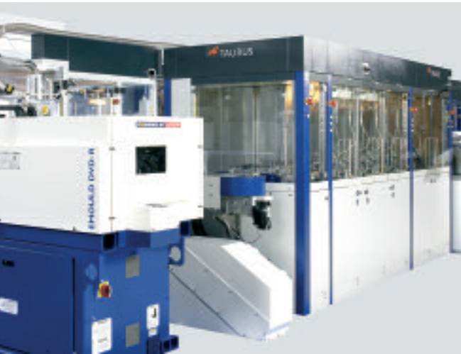
TAURUS-DVD-R replication line with EMOULD molding machine
