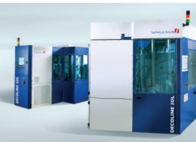
DECOLINE – Inline coating system for 3-dimensional plastic parts
