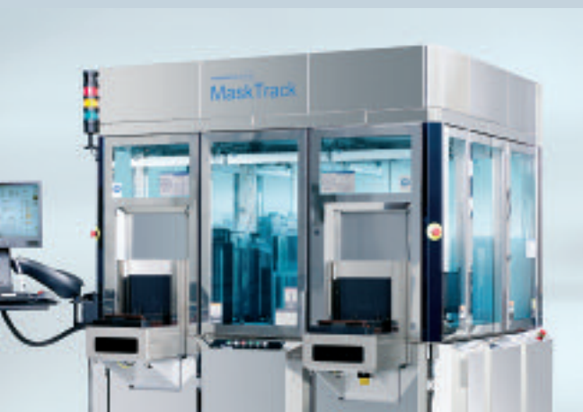
Processing system for photo mask cleaning for the semiconductor industry
