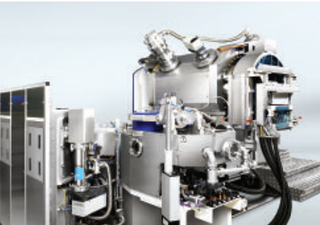
TIMARIS Coatingsystem for Read-Write-Heads and MRAM wafer
