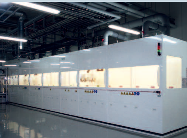
STANGL wet chemical systems, processed as "vertical batch systems", represent the foundation of an effective and competitive mass production of mono- and multi-crystalline wafers
