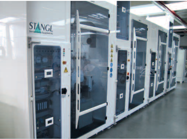
STANGL CIS/CIGS-Process system for wet chemical treatment for the thin film solar technique
