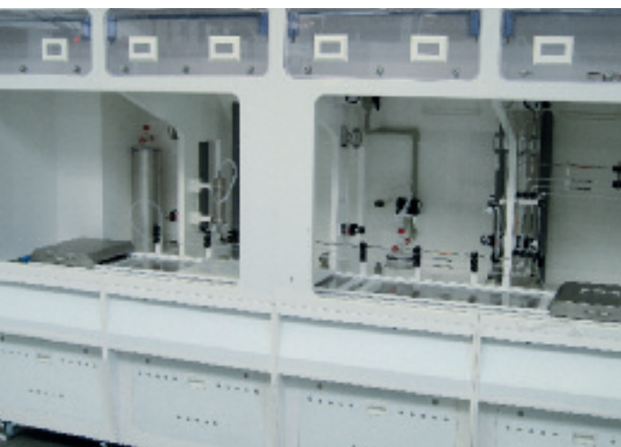
New ILGAR R&D system for the deposition of cadmium-free layers in the thin-film solar technology
