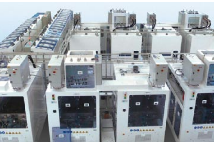
TENUIS production system for buffer layers in thin-film solar technology
