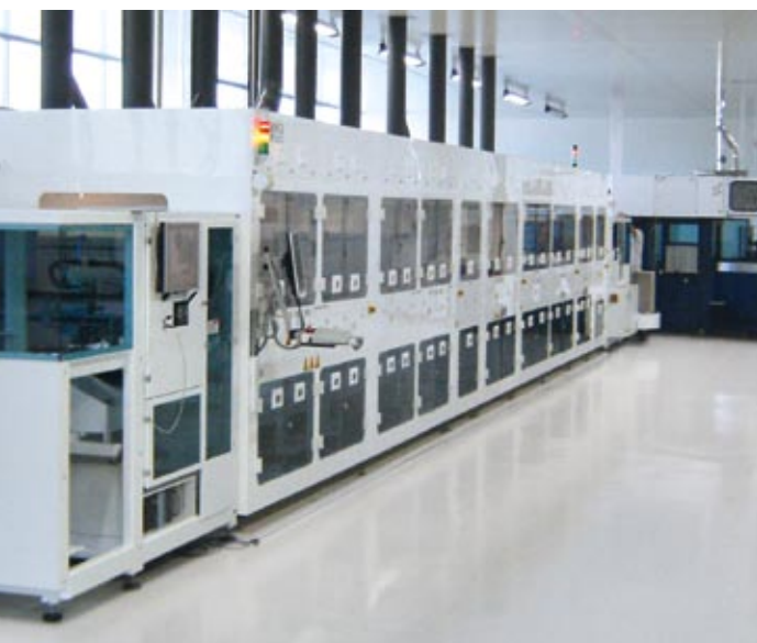
Part of a front-end production system for Si solar cells (Wafer handling, LINEA system in combination with SINGULAR)
