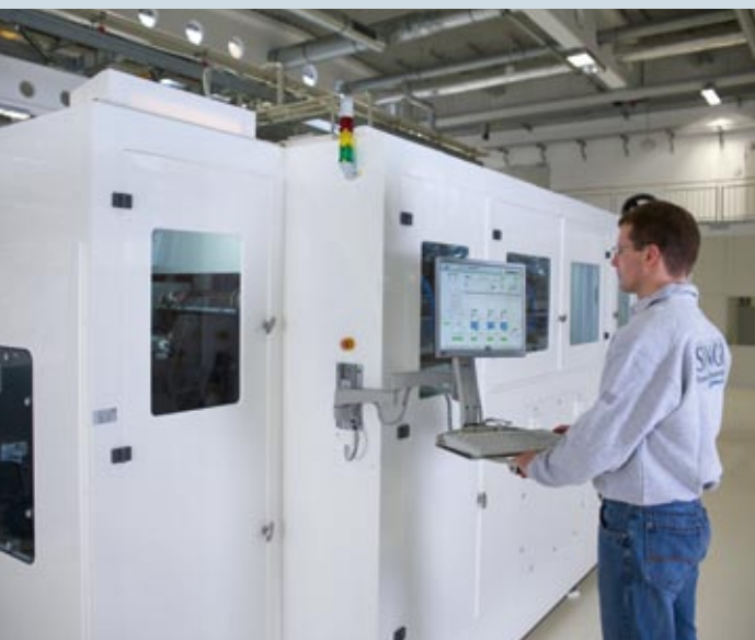
System for wet-chemical cleaning and coating of buffer layers on flexible thin-film solar cells
