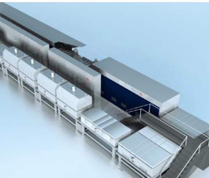
3D graphic of a diffusion furnace for thin-film solar cells
