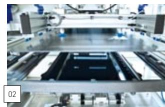
01/02 CISARIS – New system for the selenisation of thin film solar cells
