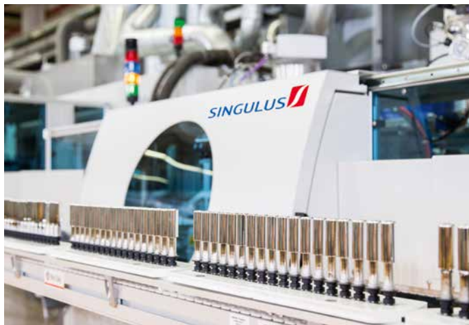
Polycoater – newly developed vacuum coating machine for decorative moulded parts, displays and touch panels
