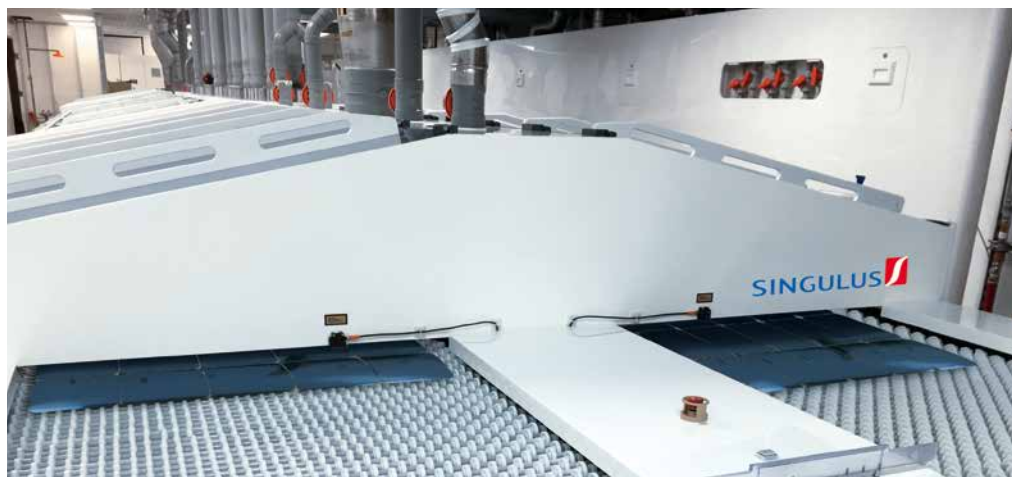
Inline system for wet-chemical processes in solar technology
