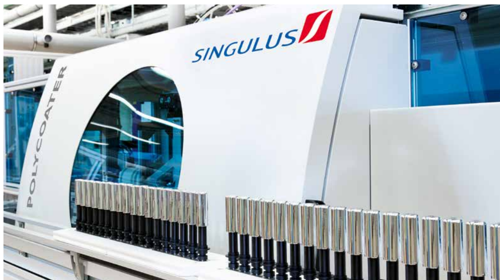
POLYCOATER: vacuum coating machine for decorative and functional layers
