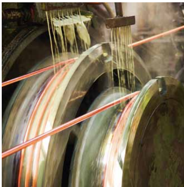
Constant cooling and lubrication is of great importance in the cold forming of copper into overhead wire.
