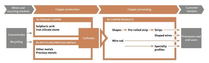
BU **Primary Copper** mainly combines the production facilities for processing copper concentrates and producing copper cathodes at the Hamburg and Pirdop sites as well as copper production at the Olen site. It also includes the production and marketing of sulphuric acid, iron silicate and other specialty products.
