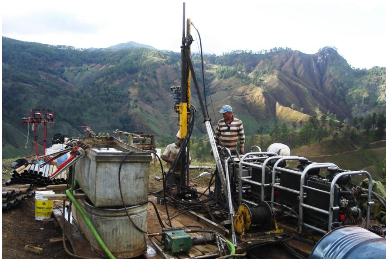
Figure 12.1 Drill rig on hole LTP-24 at Escandalosa Sur. The rig is a man-portable, hydraulic Hydracore Gopher diamond drill.
