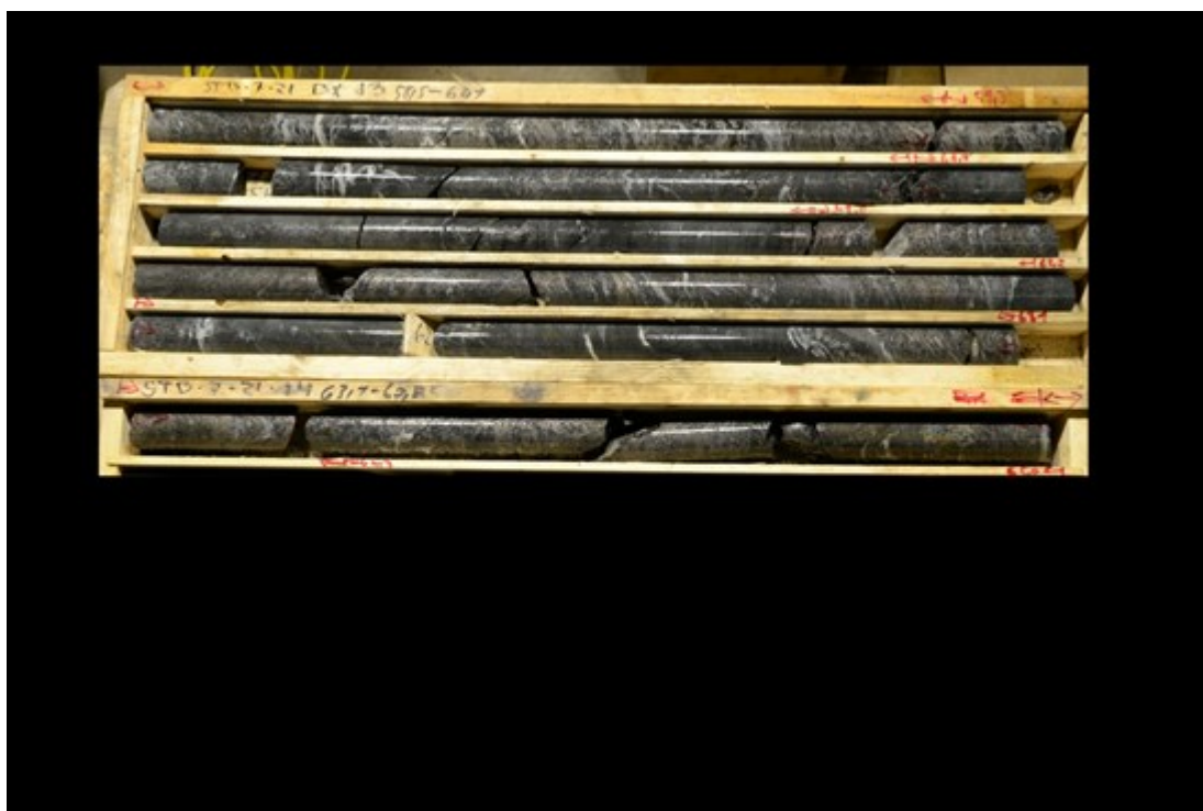
NQ core with sulphides in drillhole STB-21-007 at Storboren
