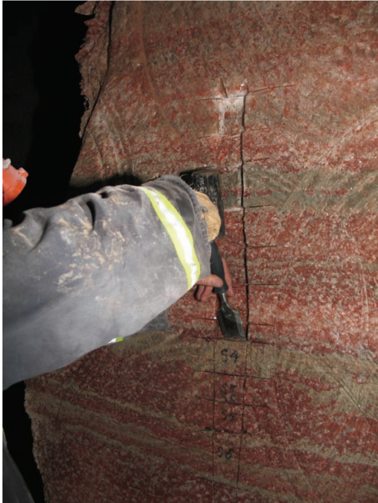
Figure 15-1: Removing Sample Blocks from the Mine Wall
