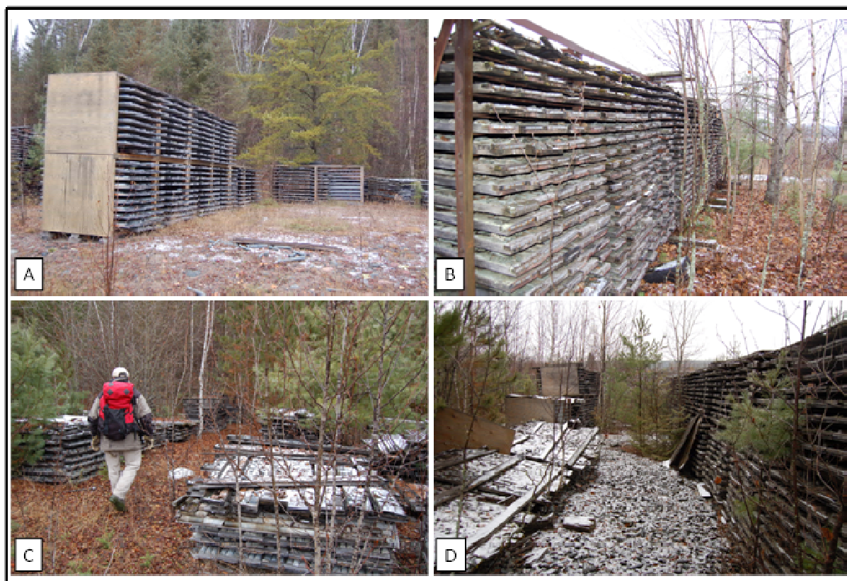
Figure 12.5 – Outdoor core storage next to the core shed: A) Recent core; B) and C) Historical core; and D) Photo showing some of the collapsed core racks.
