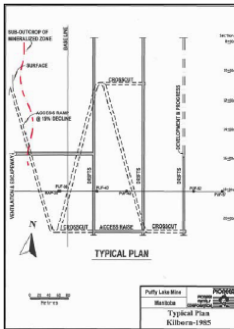
Figure 20-1. Typical Ramp Layout
