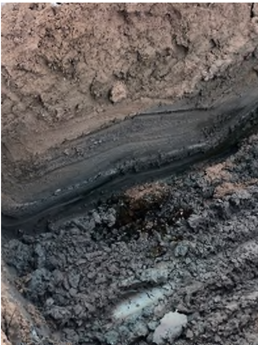
Fig 4 shows the black sands/shales unit with brine/ground water flowing into it.
