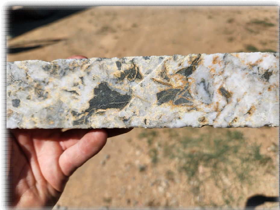
Figure 7; Framework supported breccia. Lithic are rimmed by ferro-carbonate and matrix has disseminated pyrite. Selection is from interval 113.5 - 114.25m which assayed 1.25 g/t and 4,570.8ppm As.
