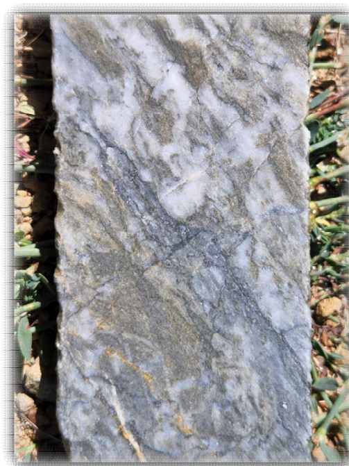
Figure 5; New reef (left) selection from high grade interval 124.450 - 125.45m in GBDD006. Sulphide and quartz veining.
