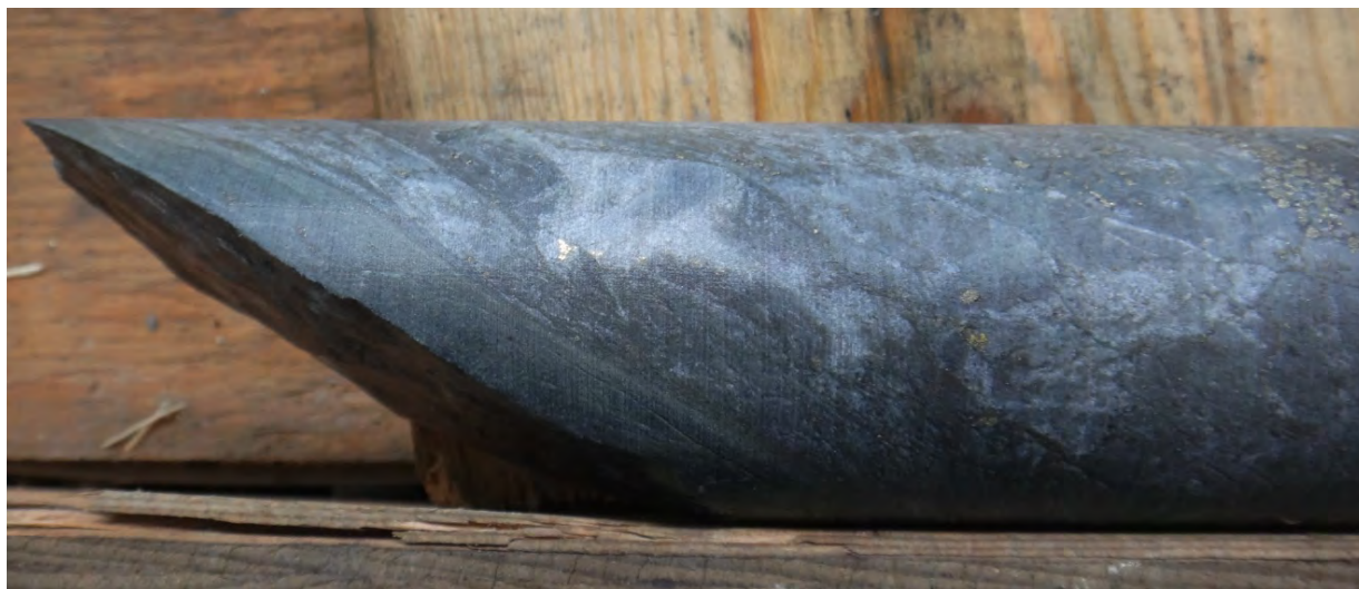
Plate 2: Visible gold occurring on the edge of a calcite + pyrite + dolomite vein hosted within moderately sheared, calcite-altered, pyritic basalt @ ~84 m in MDE-12-70 (BLFZ).
