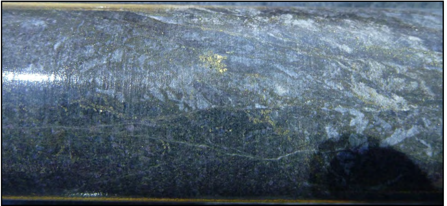
Plate 4: Visible gold at ~170.5 m of hole MDE-12-29 (Footwall Zone).
