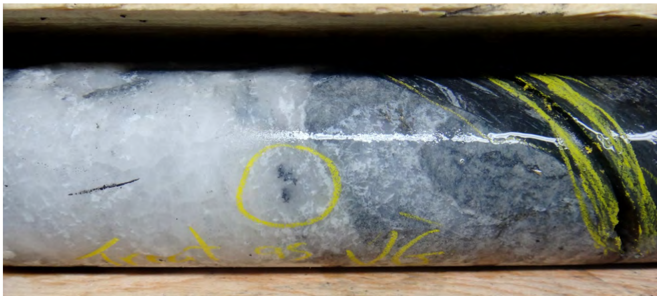
Plate 3: Unidentified grey metallic mineral (telluride?) hosted in quartz-dolomite-tourmaline vein at ~117 m in hole MDE-12-74 (BLFZ).
