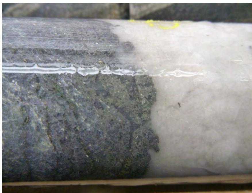
Plate 1: Coarse arsenopyrite blebs along quartz vein margin at ~254 m in hole MDW-12-55 (Martinière West).
