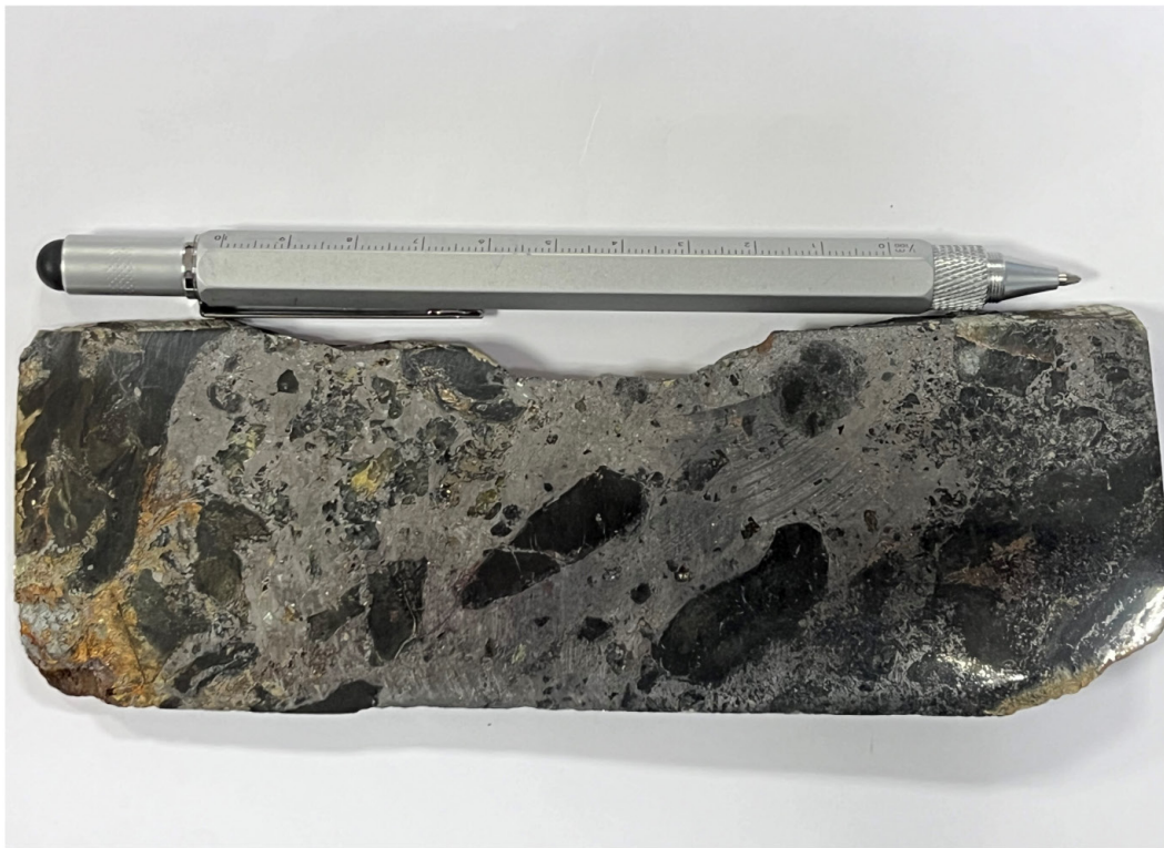
Photo 6 - Massive stibnite mineralization with metasedimentary fragments. 19.65% Sb (sample E6320458).
