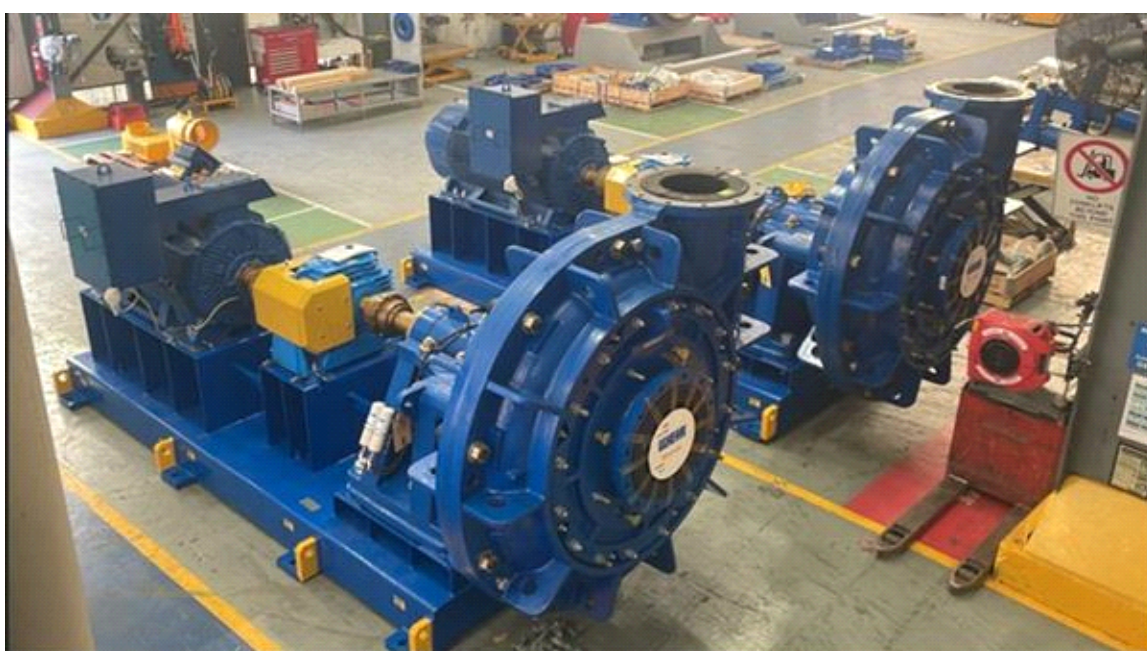
Figure 10: Cyclone Feed Pumps Ready for Collection (30 June 2025)
