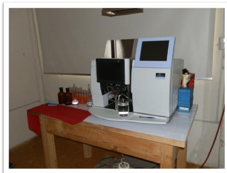
Photo 9. Goldgroup's onsite 'Perkin Elmer' Atomic Absorption Spectrometry equipment at Arroyo Agrio - Caballo Blanco Project - 2012 (Photo - Cuttle)
