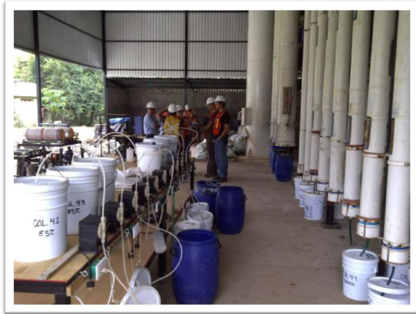
Photo 8. Goldgroup's onsite 'Column leach' laboratory at Arroyo Agrio - Caballo Blanco Project - 2012 (Photo - Cuttle)
