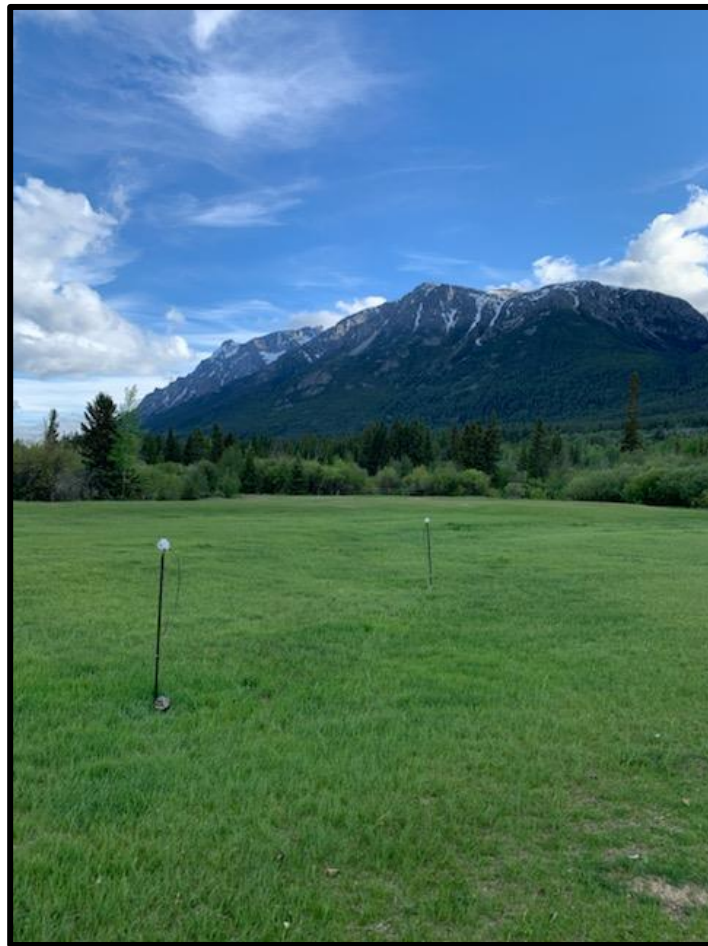
Figure 17: GEM 5 (L) and GEM 6 (R) magnetic base stations.
