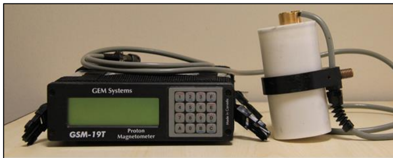
Figure 14: GEM GSM-19T proton precession magnetometer.
