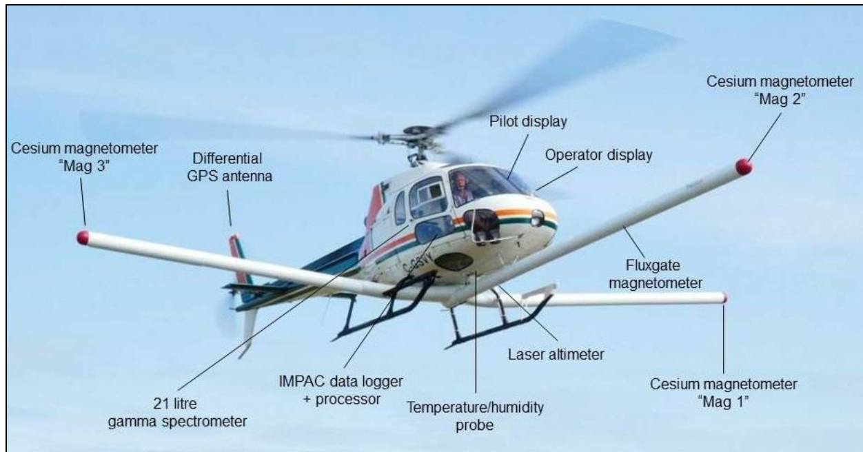
Figure 6: Survey helicopter equipped with three magnetic sensors for gradient magnetic data acquisition and gamma spectrometer.
