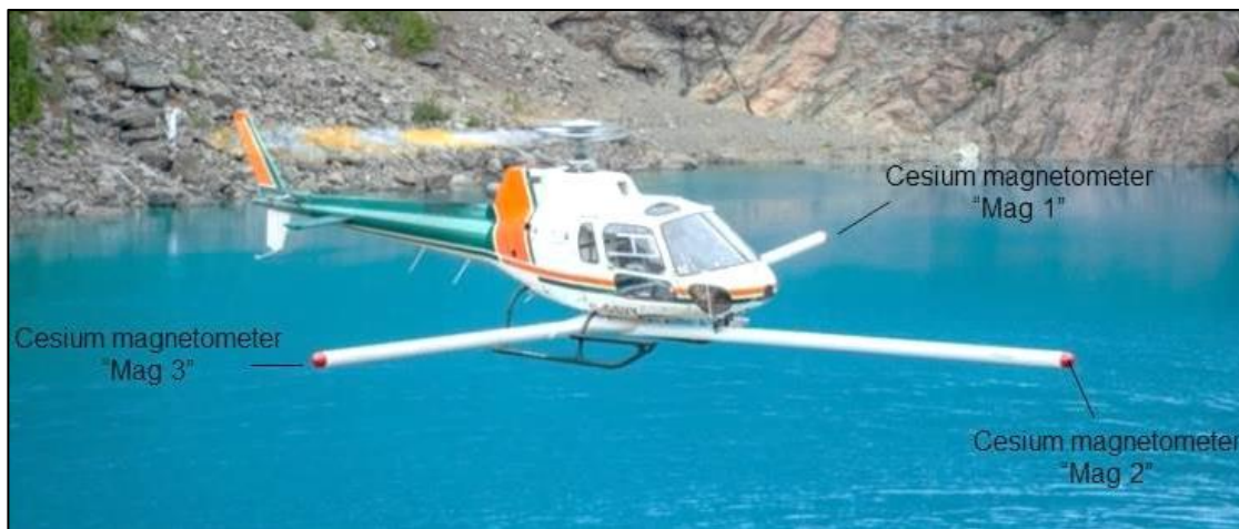
Figure 12: View of triple magnetic boom system.
