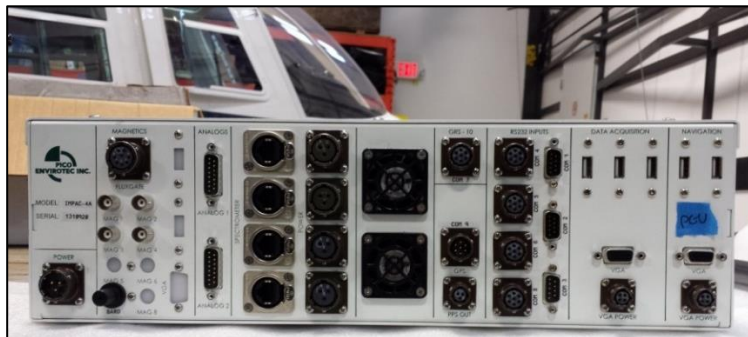
Figure 7: IMPAC data acquisition system.
