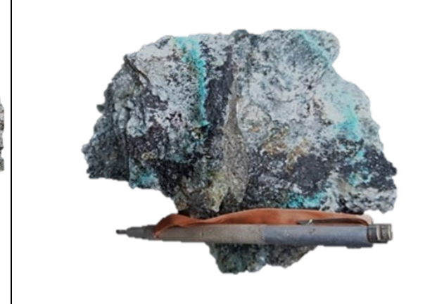
Figures 5 &amp; 6: Hydrothermal sodic-calcic breccia; magnetite-pyrite matrix and copper sulphates
