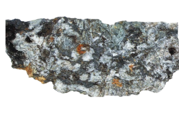
Figures 5 &amp; 6: Hydrothermal sodic-calcic breccia; magnetite-pyrite matrix and copper sulphates
